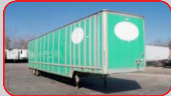
(4)1999 & 2000 Wabash 53"x102"x13'6" ALUM PLATE WALL VANS , Fixed spring ride suspension, back axles set 9' forward from rear, FRP roof, Swing rear Doors, 125" inside loading height, 101" inside loading width, 20" smooth steel scuff, 10'9" front deck, 215/75Rx17.5 tires, Hub piloted steel disc wheels, ..... $3,900 each
